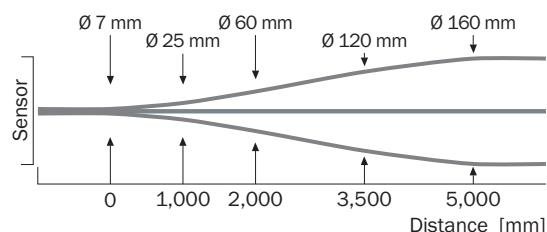
Sensing range diagram WL4S-3, WLG4S-3, 5 m
