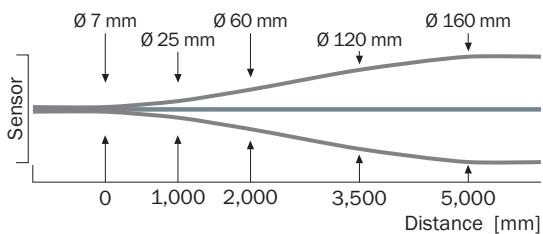
Sensing range diagram WL4S-3, WLG4S-3, 5 m
