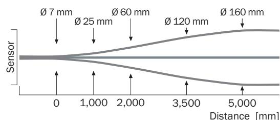
Sensing range diagram WL4S-3, WLG4S-3, 4 m
