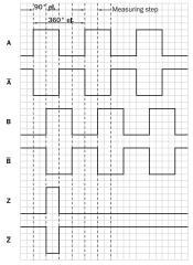
CW with view on the encoder shaft in direction "A", compare dimensional drawing.
