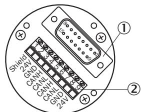
① Internal plug connector to encoder
