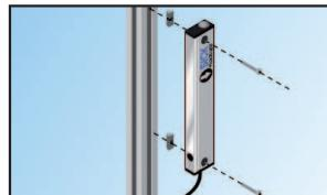
The PLG can easily be mounted on the profile with slot nuts.
