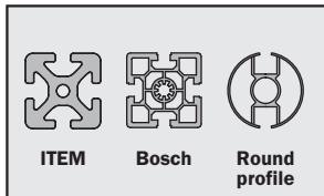
The light grid can be mounted on different profiles, e.g. ITEM, Bosch, round profile.
