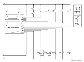
S300 Professional in connection with relays/contactors
