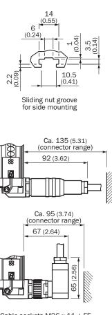
Cable sockets M26 x 11 + FE with crimp contacts
