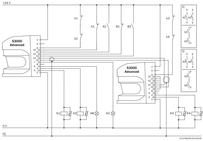
${\sf S3000}$  Advanced with  ${\sf S3000}$  Advanced in conjunction with relays/contactors
