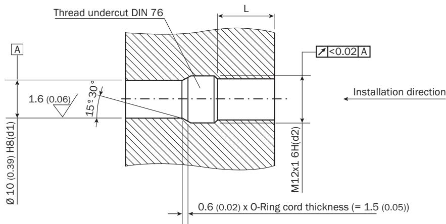
L: recommended installation depth:  $L \geq 0.8 (0.03) \times d_2$
