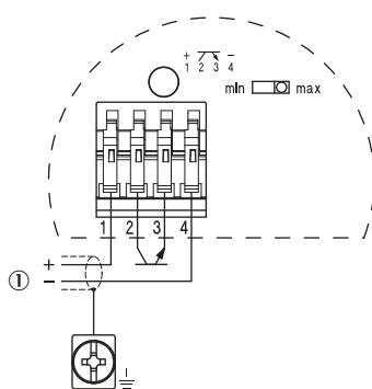
**Schéma de raccordement Comportement PNP**
