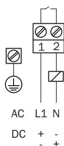
**Mode de raccordement LFV300 commutateur sans contact - Pièces électroniques**
