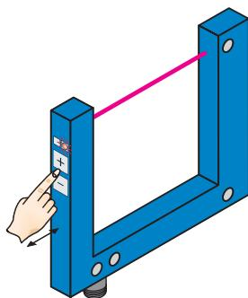
Press the “+” and “-” buttons together and hold for 1 second.
