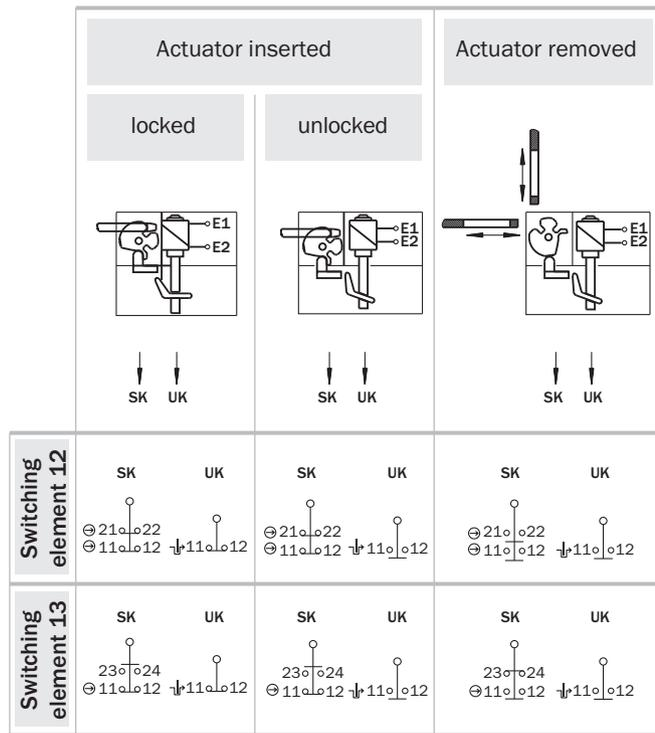
⌋ Positive action N/C locking monitoring contact
