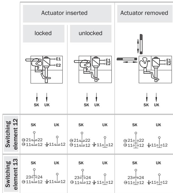
⌋ Positive action N/C locking monitoring contact
