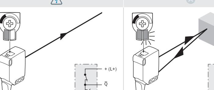
The diagram illustrates the principle of a dark switching sensor. On the left, a sensor unit with a light receiver is shown. A beam of light is emitted from its transmitter side towards a cube. The beam is interrupted by the cube, which is positioned on the right side of the diagram. This interruption causes the sensor's output state to change from HIGH (indicated by a checkmark) to LOW (indicated by a lightning bolt symbol).
