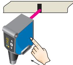
When detecting the contrast or color to be detected, "1st" flashes.
