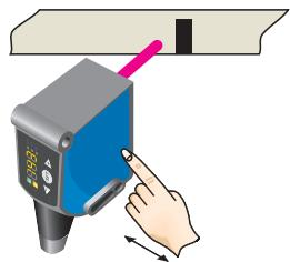
When setting the contrasts to be detected, "2nd" flashes. Press set button.
