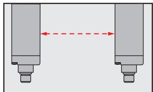
The light grid communicates via the light beams. A cable is not necessary for the optical synchronization.
