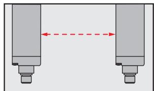
The light grid communicates via the light beams. A cable is not necessary for the optical synchronization.
