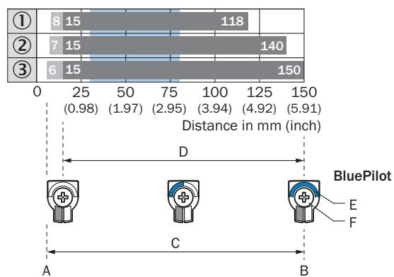
A = Sensing range min. in mm
