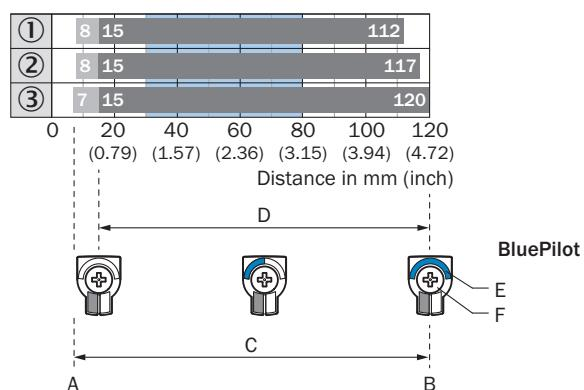
A = Sensing range min. in mm
