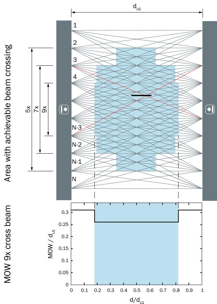
$d_{LG}$  = Installed working distance between sender and receiver
