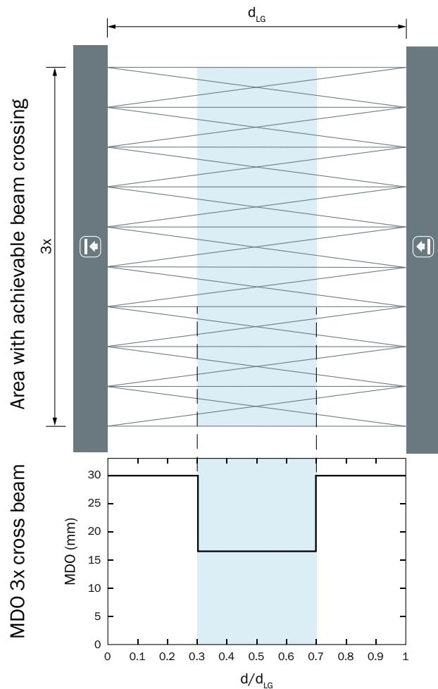
$d_{LG}$  = Installed working distance between sender and receiver
