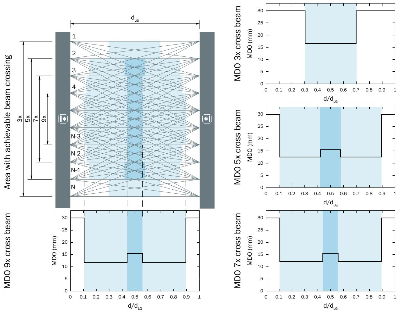
$d_{LG}$  = Installed working distance between sender and receiver
