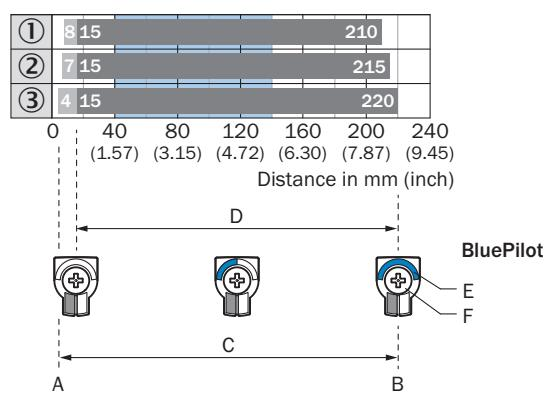
A = Sensing range min. in mm
