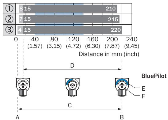
A = Sensing range min. in mm
