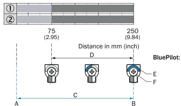
A = Sensing range min. in mm
