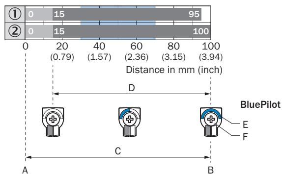
A = Sensing range min. in mm
