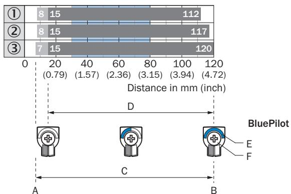
A = Sensing range min. in mm
