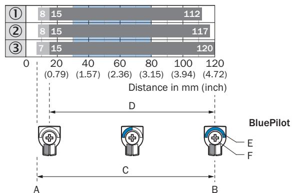
A = Sensing range min. in mm
