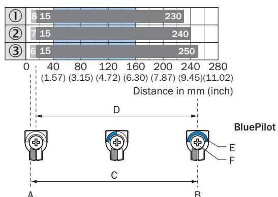
A = Sensing range min. in mm
