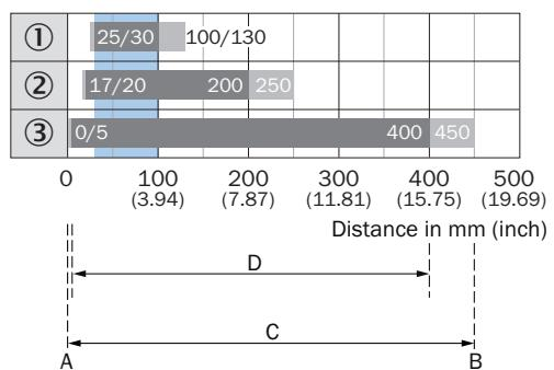
A = Sensing range min. in mm
