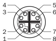
M12, prise, 8 pôles, codage X (Gigabit-Ethernet)
