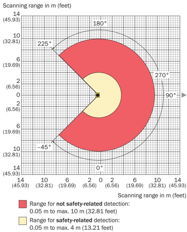
**Attention!** From the measurement origin up to a distance of 0.05 m (0.17 feet) no objects are detected (blind zone!) over the entire radial field of view (scanning range of 270°).
