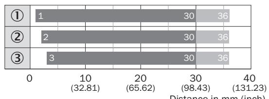
■ Sensing range ■ Sensing range max. typ.
