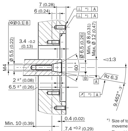
\*) Size of tolerance reduce the allowed movement of the shaft, see data sheet.
