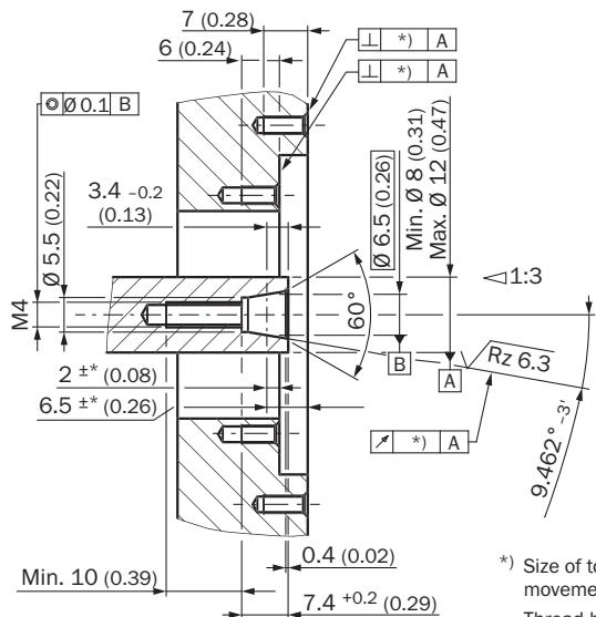
\*<sup>)</sup> Size of tolerance reduce the allowed movement of the shaft, see data sheet.
