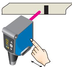
When setting the contrasts to be detected, "2nd" flashes. Press set button.
