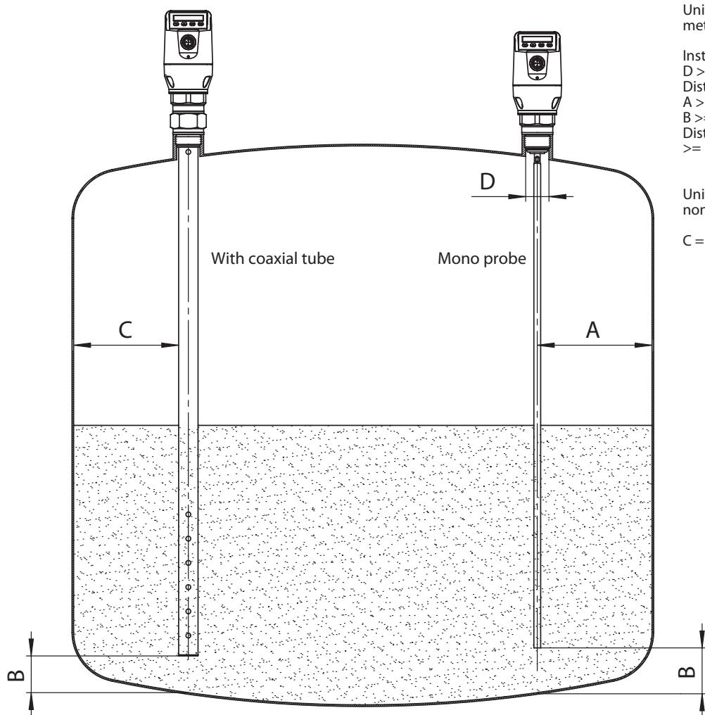
Unit with mono probe mounted in metal tank
