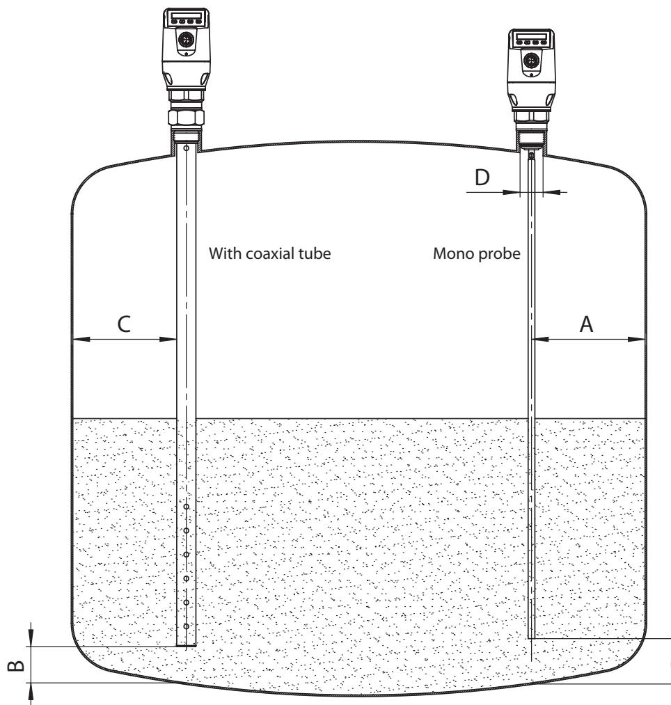
Unit with mono probe mounted in metal tank
