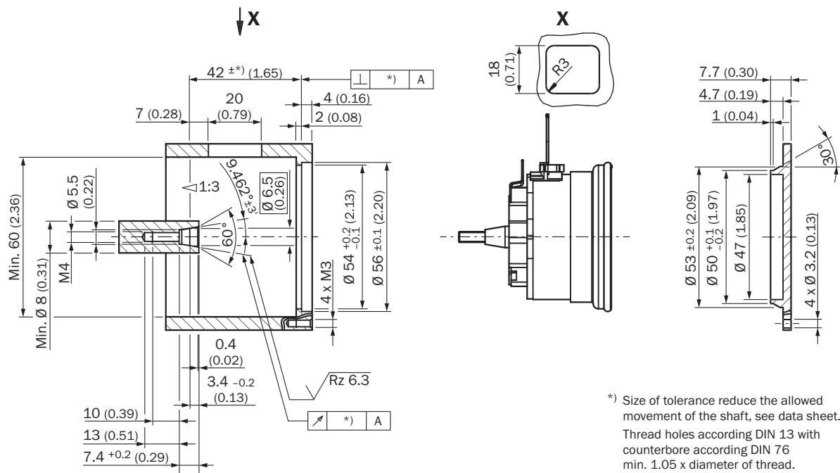
\*) Size of tolerance reduce the allowed movement of the shaft, see data sheet.
