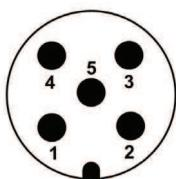
View to the connector M12 fittet to the encoder body
