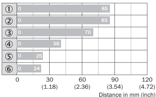
Max. sensing range S<sub>n</sub>, flush or non-flush installation,
