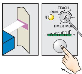
Turn rotary switch to "+" position and press and hold teach-in button until yellow light goes out (more green LEDs illuminate on the bar display).
