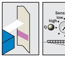
If yellow LED illuminates, turn "Sensitivity" rotary switch counter-clockwise until the yellow LED just goes out.
