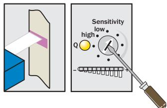
Turn "Sensitivity" rotary switch clockwise until yellow LED illuminates.
