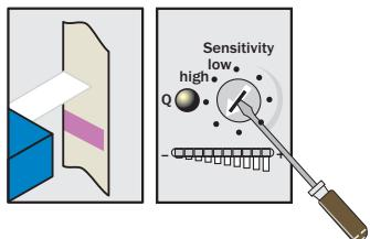
If yellow LED illuminates, turn "Sensitivity" rotary switch counter-clockwise until the yellow LED just goes out.
