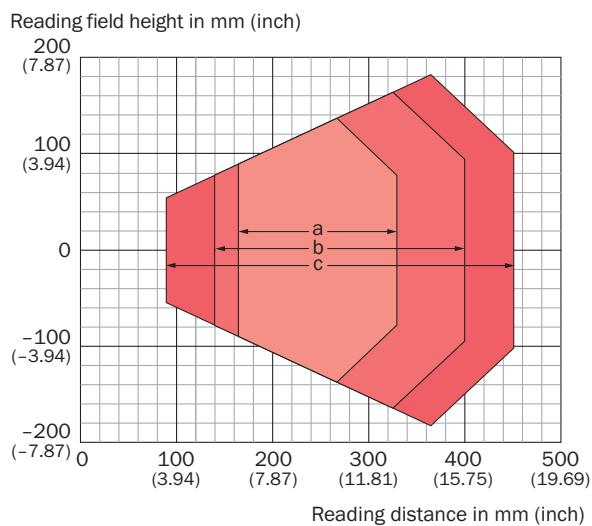
For devices with plastic reading window, the depth of field is reduced by approx. 10 %.
