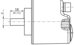
Dimensions in mm (inch) diameter x f7 corresponds to the shaft diameter
