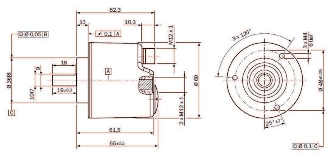
Dimensions in mm (inch) diameter x f7 corresponds to the shaft diameter
