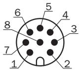
M12 male connector, 8-pin, A-coded
