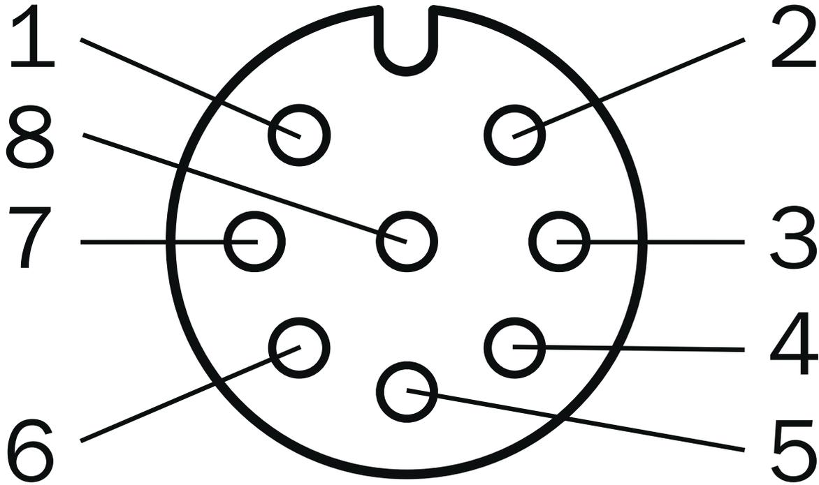
female connector M12, 8-pin, A-coded
