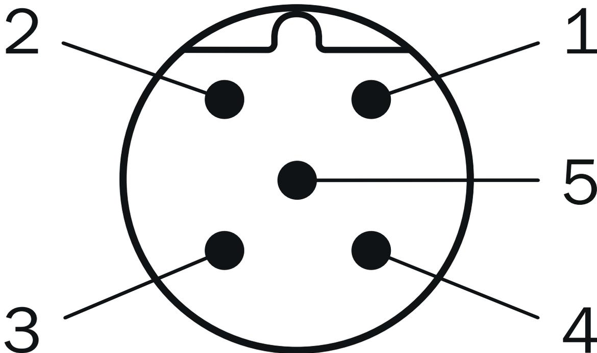
male connector M12, 5-pin, A-coded
